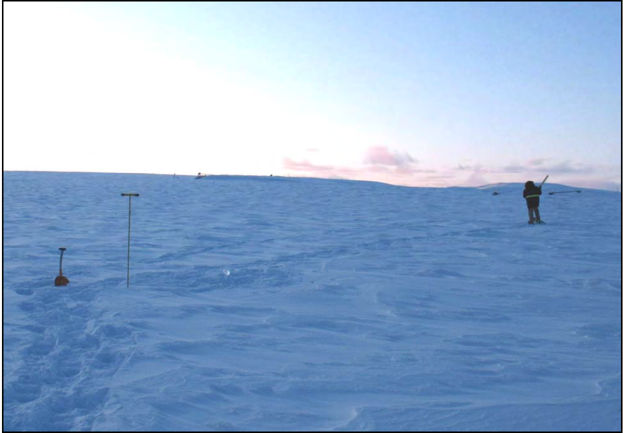
Figure 2. Jeff Derry collecting snow density samples along snow course, T-handle probe for measuring snow depth in foreground, Toolik Lake NRCS index site. Photo by Michael Lilly, November 21, 2009.
