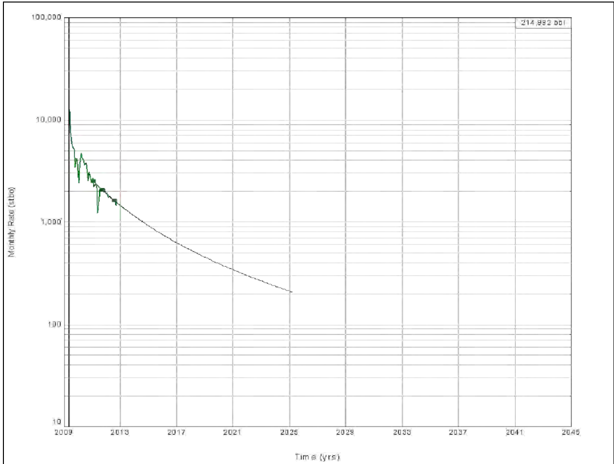
Decline curve analysis for the ZZ 99-34H well located in Section 34, T. 99 N., R. 99 W.
