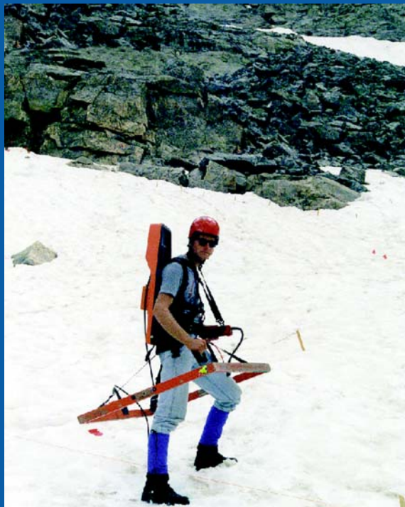
Figure 18 – EMI skirt configuration. Photo courtesy of Blackhawk Geometrics.
