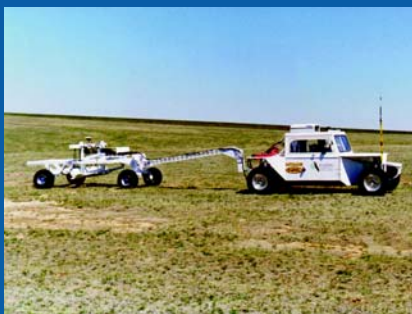
Figure 13 – Multisensor Towed Array Detection System (MTADS) configured with cesium vapor magnetometers. Photo courtesy of Blackhawk Geometrics.
