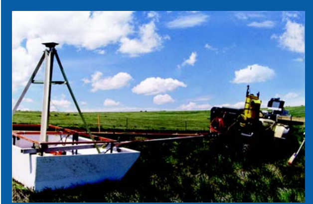
Figure 22 – Ground penetrating radar sled in towed configuration. Photo courtesy of Blackhawk Geometrics.
