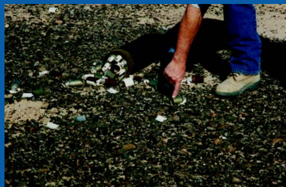
Figure 30 – A 155 mm artillery dispenser carries grenade-like submunitions to the target. This dispenser did not open properly to scatter the submunitions; the inert submunitions fell out when the round hit the ground. Submunitions are small and often do not look like military munitions.
