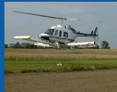
Figure 15 – Helicopter configured with magnetometers for UXO and DMM detection. Photo courtesy of Oak Ridge National Laboratory.
