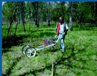
Figure 14 – Cart system configured with cesium vapor magnetometers. Photo courtesy of Blackhawk Geometrics.
