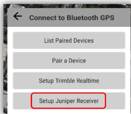
Setup Juniper Receiver with Bluetooth
