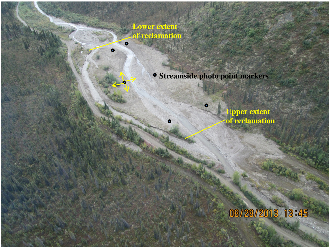
Figure 3. Establish a minimum of 6 photo points along the stream to monitor change over time. Four photos should be taken (downstream, across, upstream, 180° away from stream) annually from each photo point.
