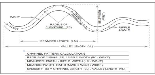
Figure 1. PATTERN MEASUREMENTS AND RATIOS, INCLUDING THE MEANDER WIDTH\*
