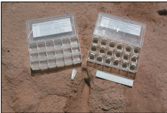
Figure 8.10. Complete soil stability kit with water and samples.
