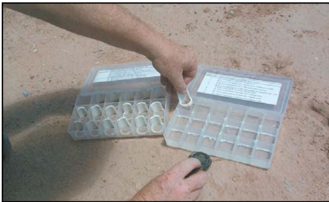
Figure 8.9. Place first sample in water.
