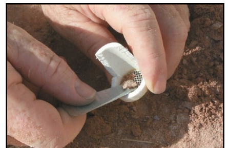
Figure 8.3. Place sample in sieve.
