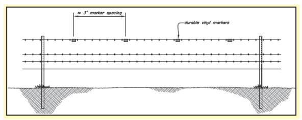
[NOTE: This diagram displays the proper placement of the fence markers. For an "exclosure" fencing design, refer to the BLM/FS Oil and Gas Gold Book - Exclosure Fence Illustrations, Figure 1.]
