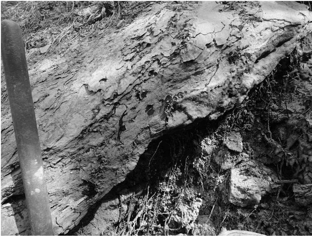
Figure 6. Asphalt impregnated rock located along same flow path in gulley as recent spill (UTM 436299E, 4162055N). Heavy exfoliation of the asphalt impregnated rock surfaces indicate it is probably more than 10 years old.
