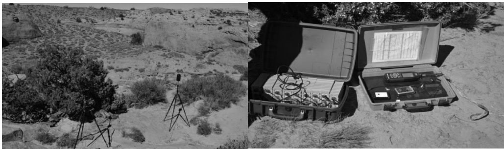
Dry Fork acoustic monitoring station equipment includes a microphone, digital recorder, sound pressure level (dB) meter, a weather station, and batteries.
