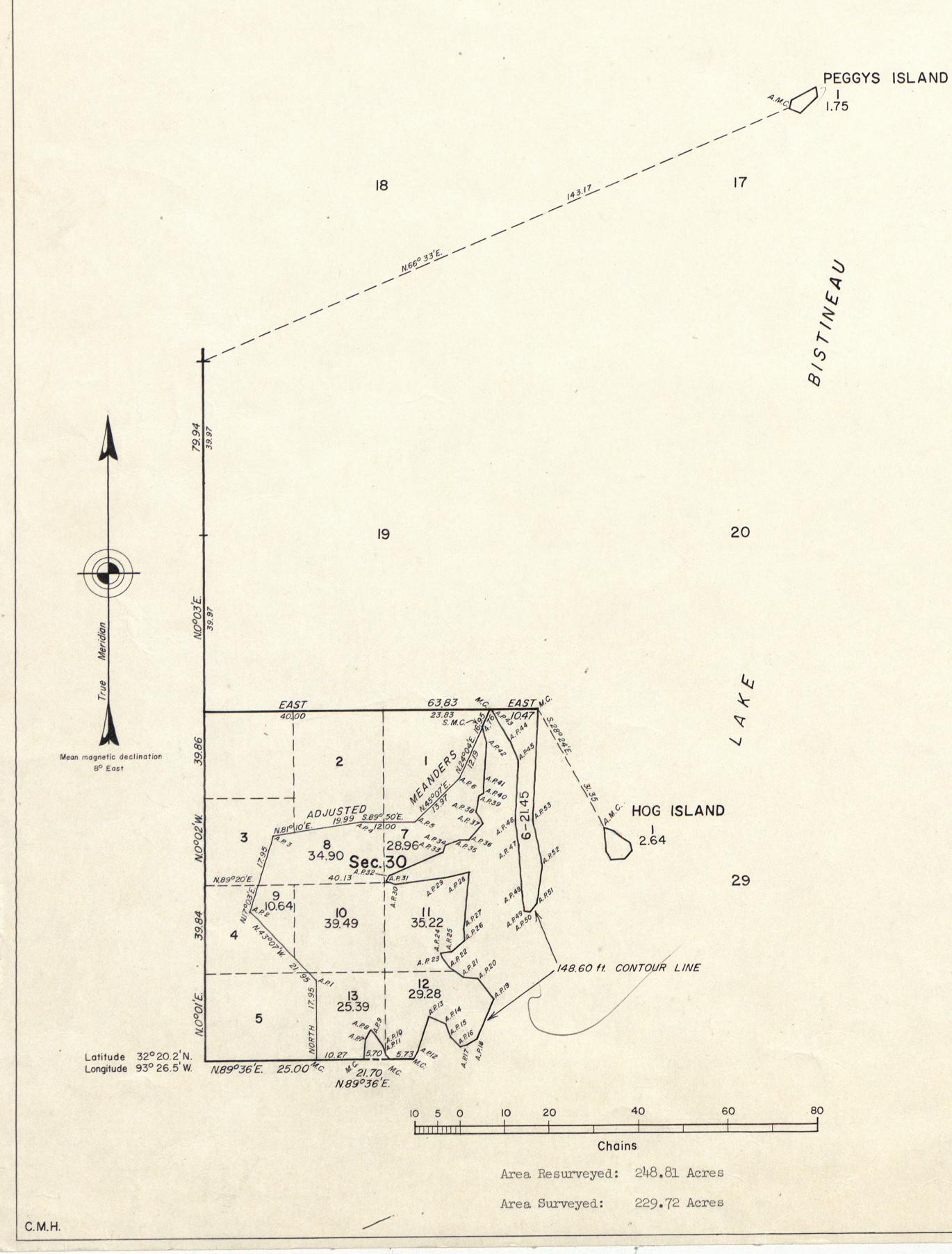
This plat represents a retracement and reestablishment of a portion of the west boundary and subdivisional lines, designed to restore the corners in their true original positions according to the best available evidence, and, an extension survey in section 30, the survey of Peggys Island, section 17, and Hog Island, section 29.
