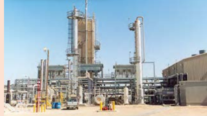
Crude helium enrichment unit in the Cliffsides Gas Field.
