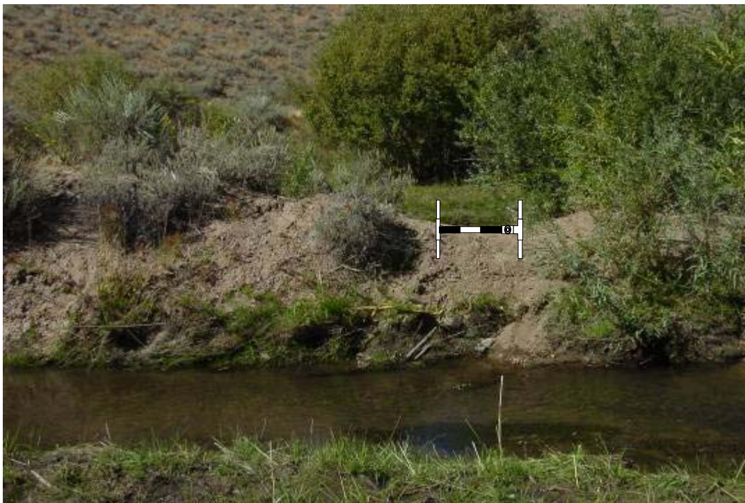
Figure 48 —a narrow peninsula on a tight meander bend has no greenline vegetation. Place the frame with the center bar along the top of the ridge and record “NG” (no greenline vegetation). Record the applicable data.
