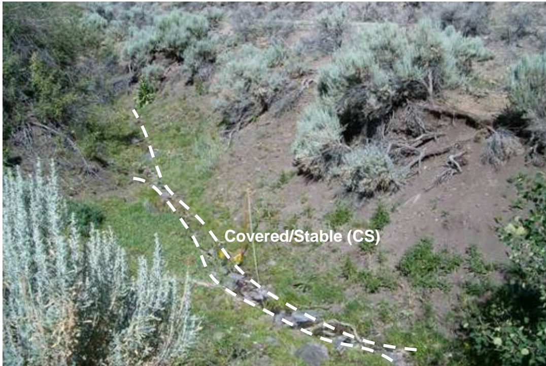
Figure 9 —the scour line and greenline are at approximately the same location. The streambank has at least 50 percent vegetation cover and is not eroding. Thus is classified as covered/stable (CS). Photo- PIBO, U.S. Forest Service.
