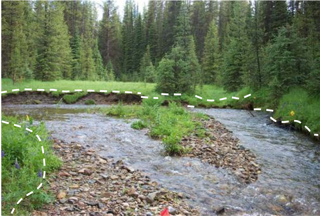
Figure 19 —the island, even with vegetation is not part of the greenline. The slump blocks on the far bank are not counted as greenline because they still in a non-stable state. Photo - PIBO, U.S. Forest Service
