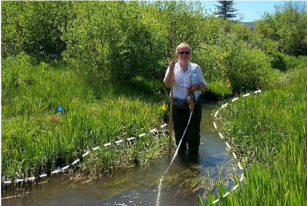
Figure 9 —greenline follows the continuous vegetation along the edge of the water at summer low flow and not vegetation growing in the water or channel. There is a distinct line between the vegetation on the streambank and the vegetation in the channel. Photo - PIBO, U.S. Forest Service
