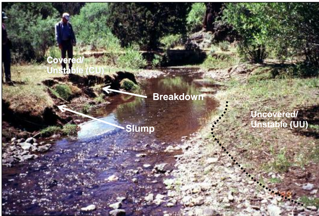
Figure 20 —the left bank contains slumping banks and breakdown is covered/unstable (CU). The right hand bank is a point bar with less than 50 percent vegetative cover. The condition of the right bank is uncovered/unstable (UU).
