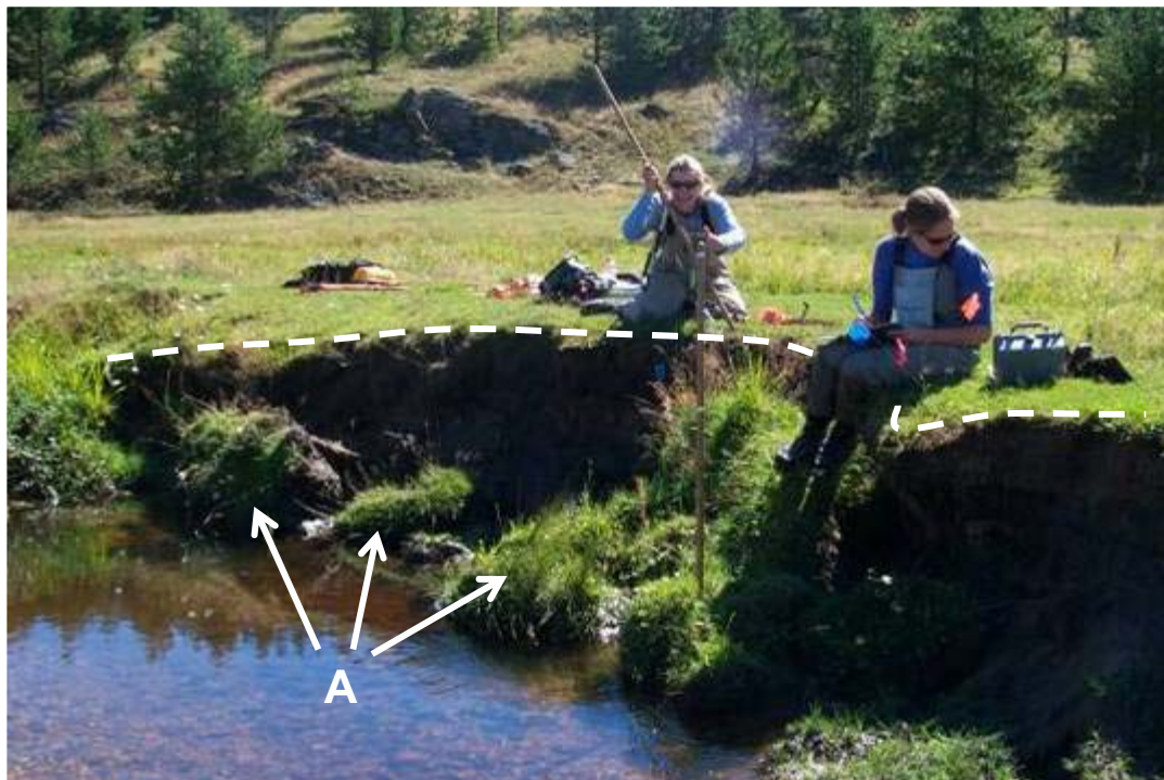
Figure 24 —slump blocks “A” are detached and not considered part of the greenline. The dashed line shows greenline. Photo - PIBO, U.S. Forest Service
