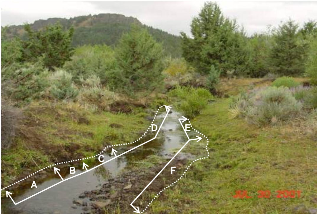
Figure 21 —the dotted line in the scour line. “A” has bare bank above the scour line with vegetation on top (covered/unstable (CU)). “B” is uncovered/unstable (UU). “C” is covered/unstable (CU). “D and E” has a vegetation cover with little erosion, covered/stable (CS). And, “F” is covered/unstable (CU) as a result of livestock trampling.
