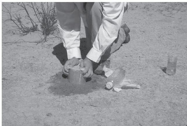
Figure 8.4. Insert infiltration ring to 3 cm.
