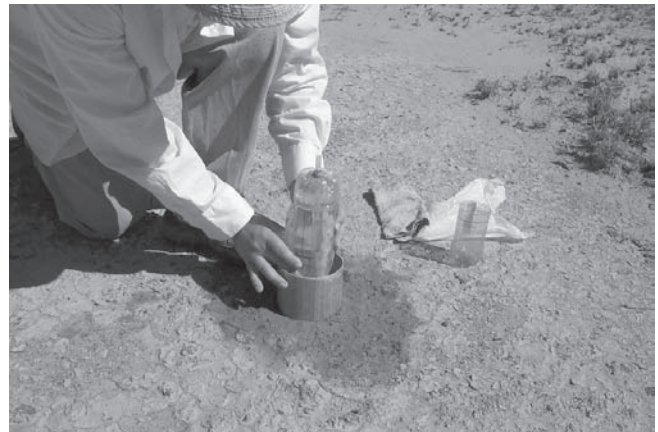
Figure 8.7. Suspend bottle inside the ring.
