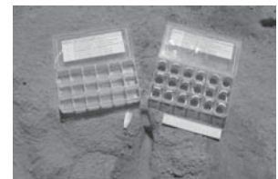
Soil stability test
