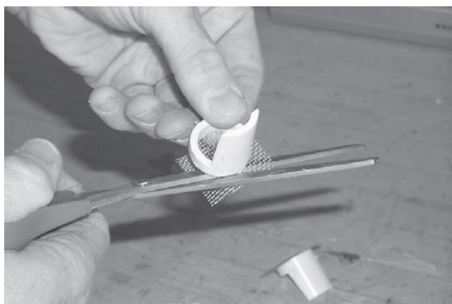
Figure A.4. Cutting out baskets from screen.
