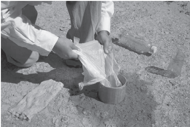
Figure 8.5. Add 370 ml water, using plastic sheet.
