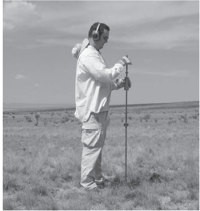
Figure 7.1. Impact penetrometer with sliding hammer elevated.
