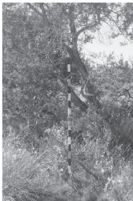
Figure 11.2. Example of a cover pole with some visual obstruction.
