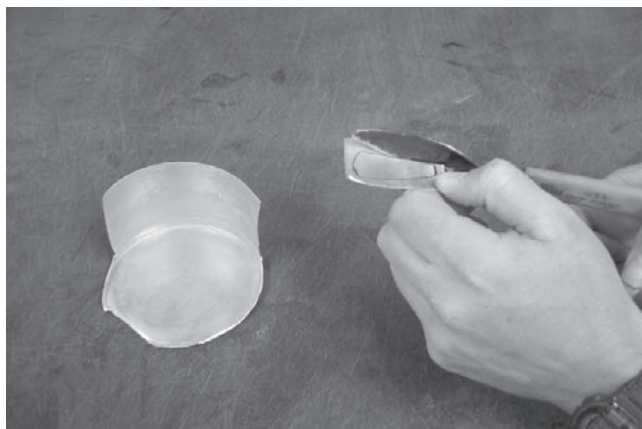
Figure A.5. Cutting shovels with tin snips.
