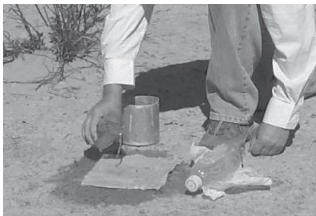
Figure 8.3. Pre-wet the soil to a 4 cm depth.
