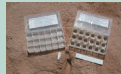
Soil stability test
