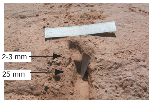
Figure 17. Excavate trench for subsurface sample.
