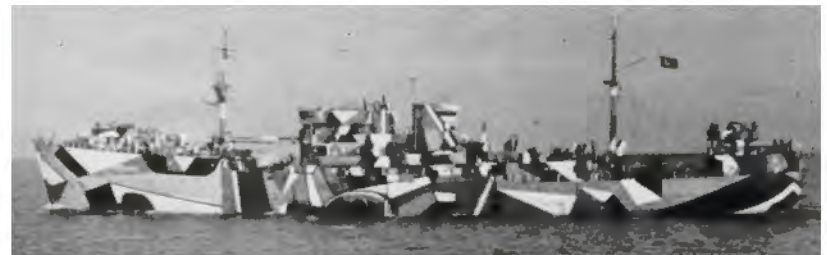
Examples of dazzle painting used on warships in World Wars I and II.
