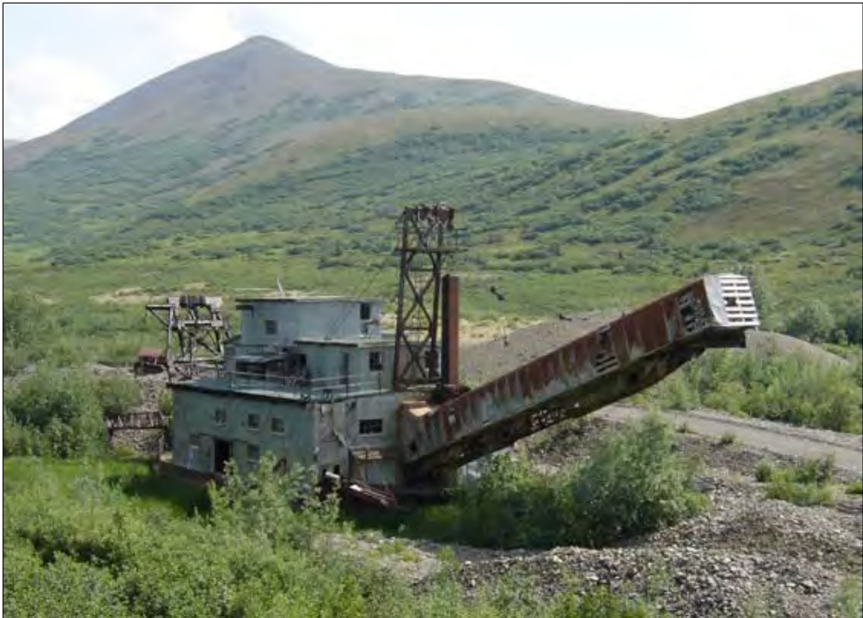
Figure 27. Inactive bucket-line dredge on upper Bear Creek, a tributary of the Tuluksak River; dredges operated on this drainage almost continuously from 1925 to 1988
