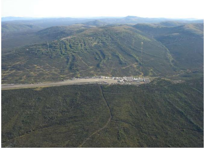
▲ Figure 16. Aerial view looking East at the Donlin Creek site. Camp facilities and airstrip are on the foreground. A stockwork of gold-bearing quartz veinlets underlies the ridge on the far side of the airstrip.
