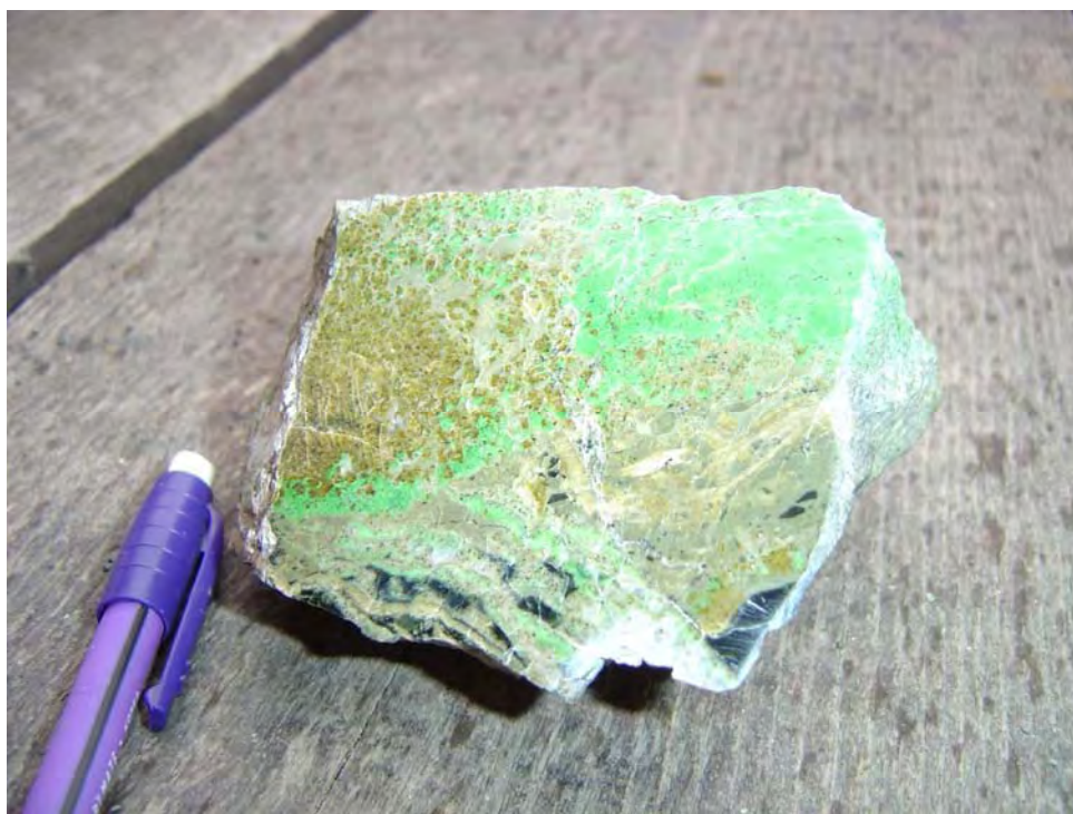
Figure 33. Polished hand sample from the Green Wonder occurrence. The olive green is garnet and the bright green is chrome diopside.
