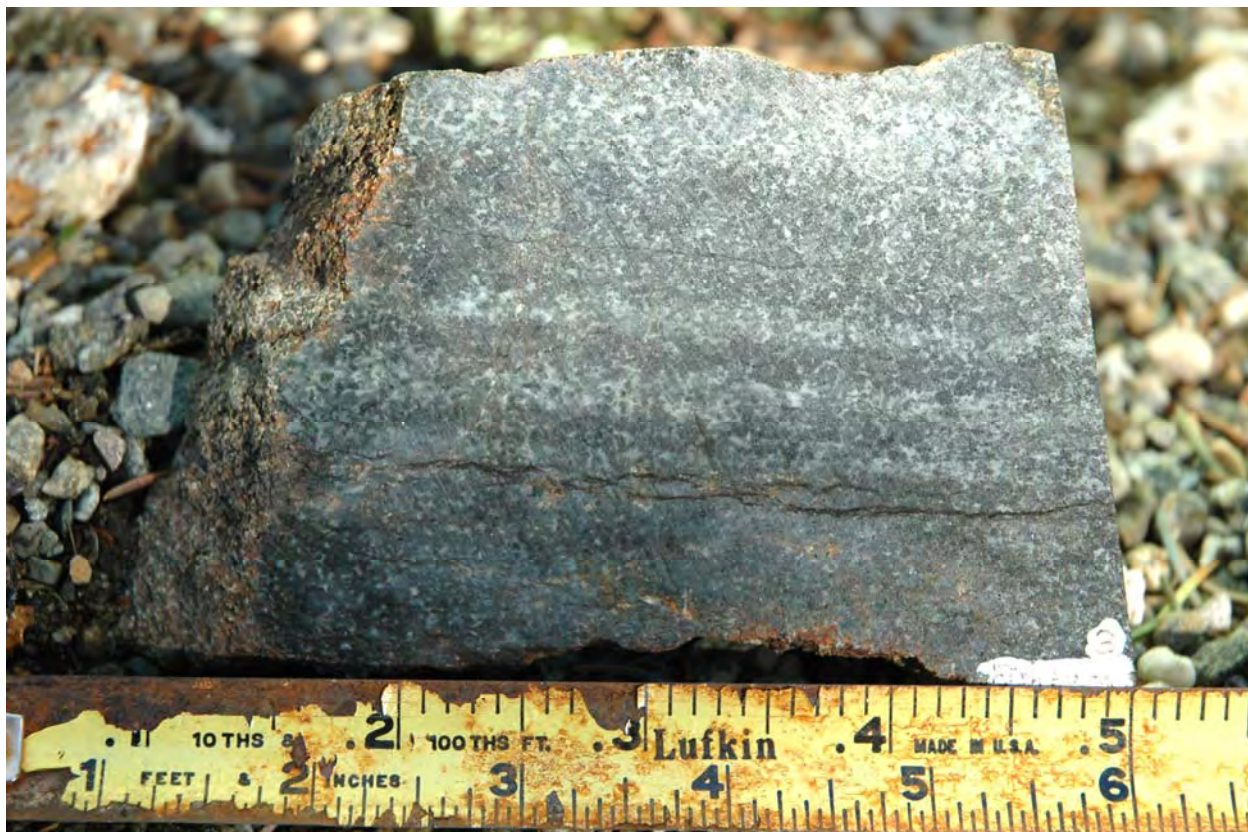
Figure 29. Layering defined by compositional variations in Fish Lake gabbro.
