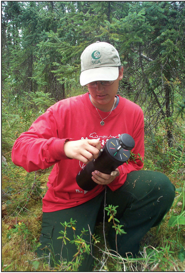
Figure 15. Technician J. Hrobak measures duff moisture with handheld DMM600 (Campbell Scientific, Inc.).
