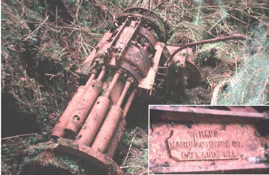
Photo 14. Ruins of a ten-stamp Straub mill that was installed at the Maid of Mexico Mine during the 1920's. Inset shows the manufacturer's plate. Photo by J. Still.
