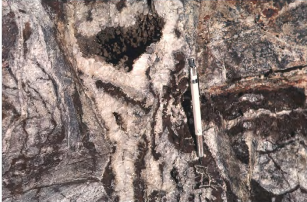
Photo 30. Silicified, vuggy, crosscutting vein from the north end of the Huff prospect. The vein pinches and swells and includes irregular lenses of silver-bearing galena. Photo by M. MacDonald.
