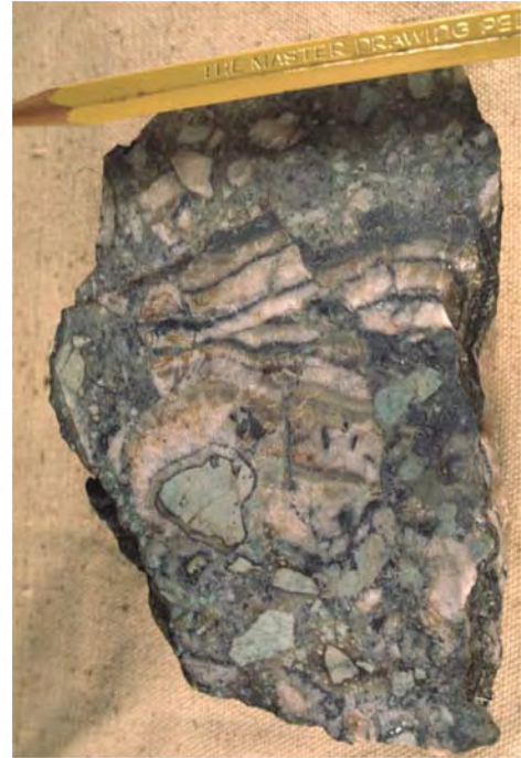
Photo 5. Mineralized breccia of green tuff. Seams and disseminations of galena and sphalerite with pink barite. Photo by P. Bittenbender.
