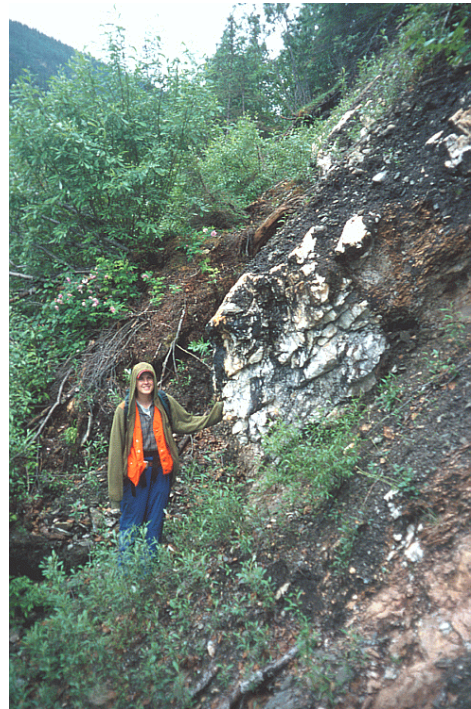
(Left) Figure 13. Fractures in phyllite containing gold-bearing quartz veinlets near Friday 13 th Pup. Samples contain up to 63.6 ppm (1.86 oz/ton) gold (map no. W90).
