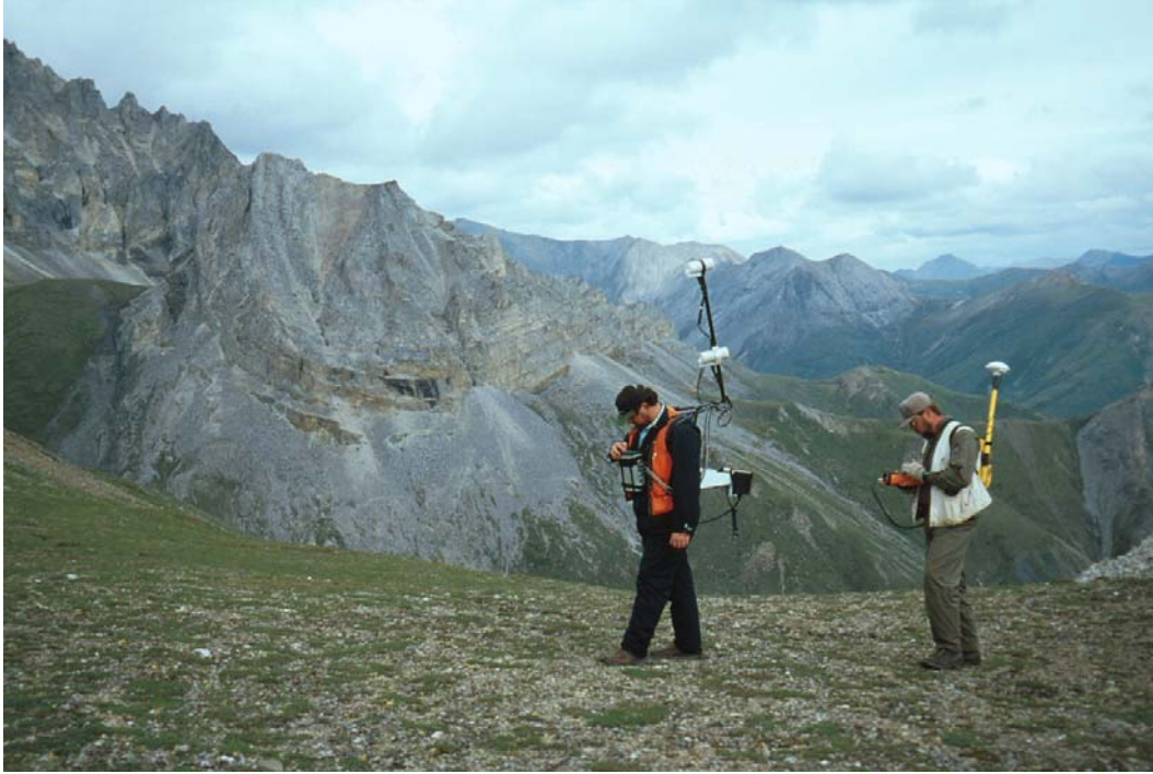
Figure 7. Ground magnetic and VLF survey, near the Ginger prospect (map no. C17), Big Spruce Creek.
