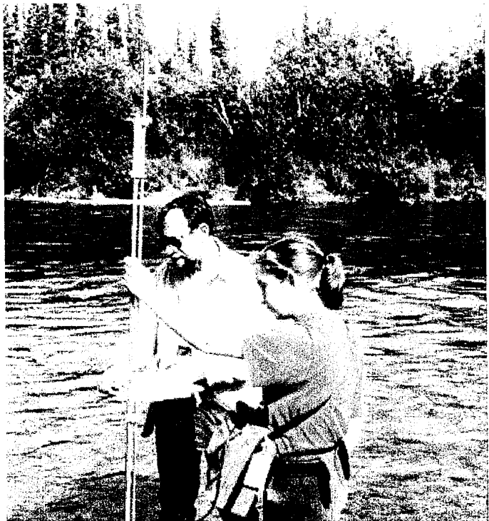
Photo 5. Standard discharge measurement techniques were used during this instream flow assessment.
