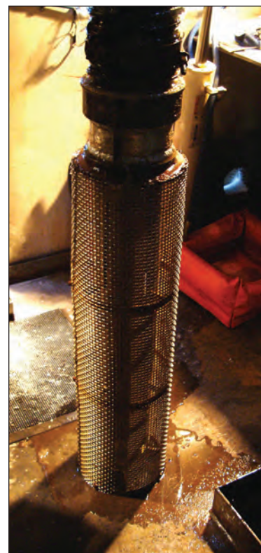
Figure 5. Intake screen being checked for proper use and condition.
