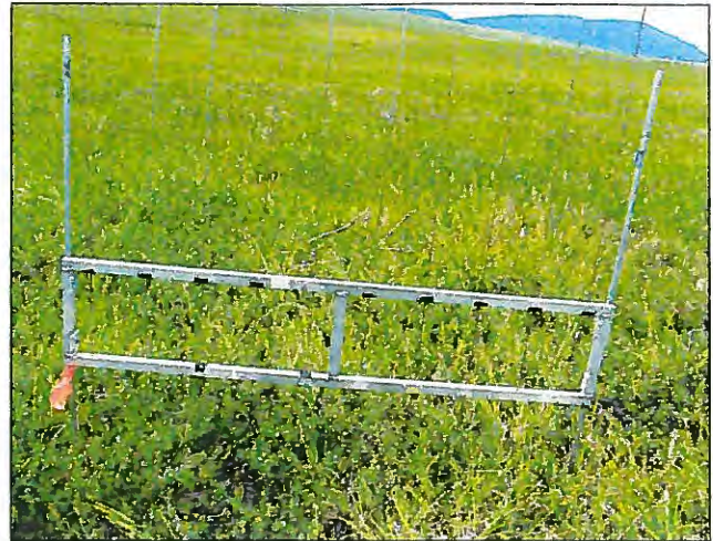
Figure 4. Vertical point frame used to measure tundra disturbance in the Toolik Lake ACEC, Alaska, 2007. The frame is 1 m long and has 10 pins spaced at 10-cm intervals along the frame.
