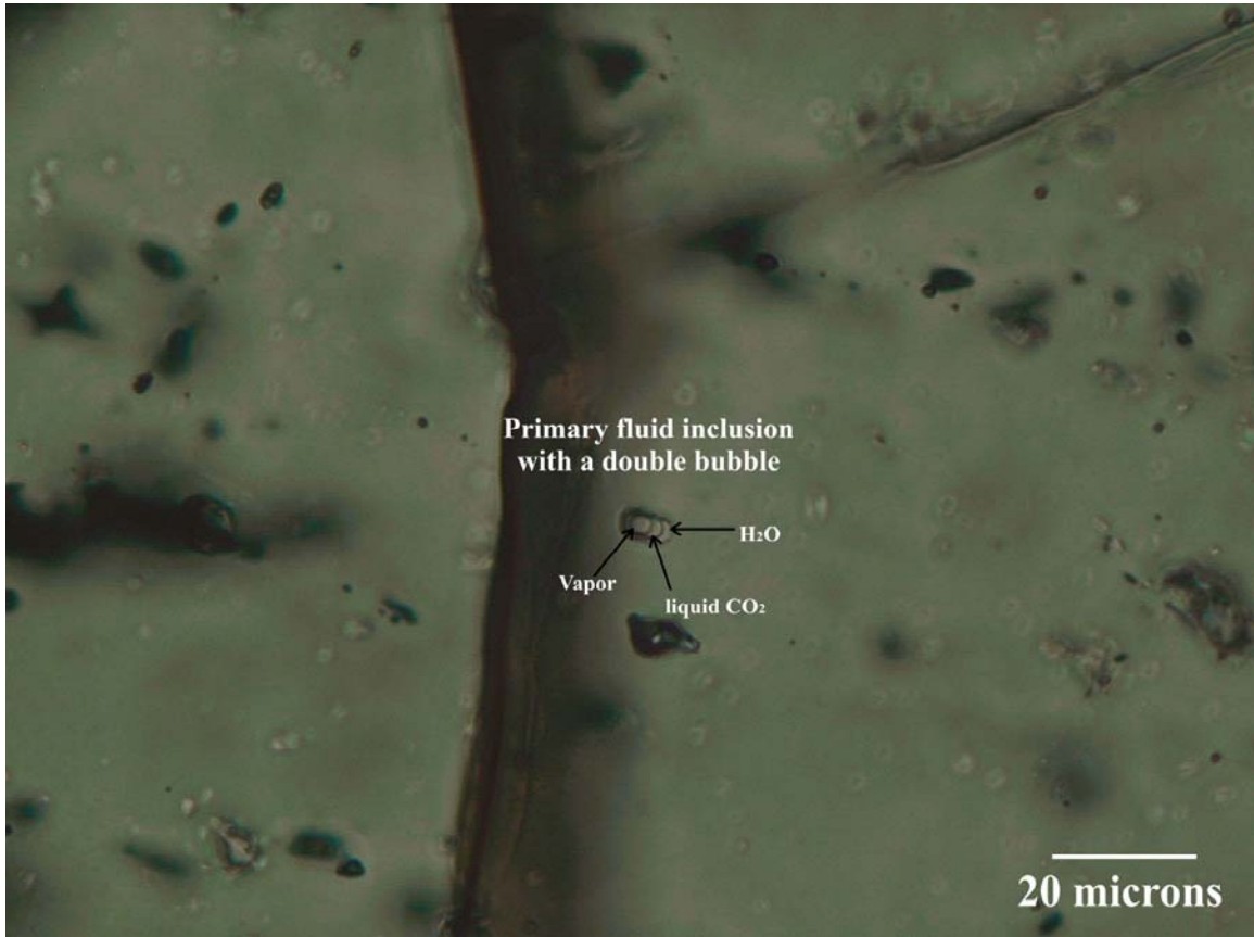
Figure 3.5: Fluid inclusion in mineralization associated quartz veining from the Wallace occurrence. Double bubble is due to the presence of water and liquid CO 2 . Sample 03ZW369.
