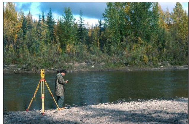
Figure 5. While most surveying employed a level and stadia rod, multi-cross-section surveys were often done with a total-station theodolite.
