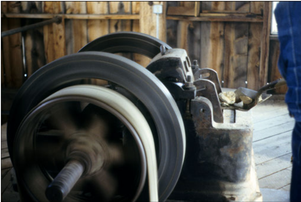
Figure 3.27. Jaw crusher in operation, Western Museum of Mining & Industry, Colorado Springs, Colorado, 1996 (photograph by Karen K. Swope).
