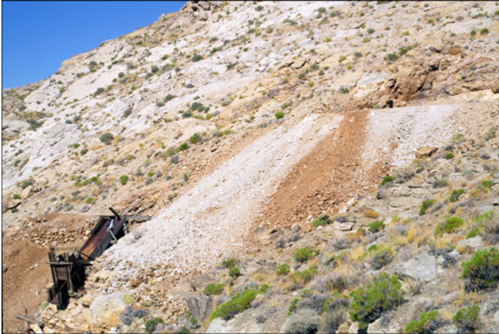
Figure 3.17. Waste-rock dump, Chloride Cliff, Death Valley National Park, 1998 (photograph by Karen K. Swope).
