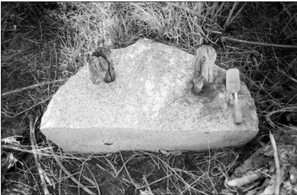
Figure 3.23. Arrastra drag stone, Beveridge Mining District, Inyo County, 1991 (photograph by Karen K. Swope).
