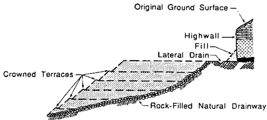
Cross Section of Typical Head-of-Hollow Fill.
