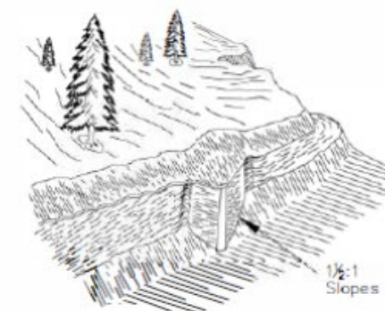
Typical Culvert Removal – After
