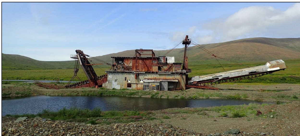
Figure 2: Yuba diesel electric dredge where it sank in 2005 on the Salmon River near the confluence with Medicine Creek. The base of Red Mountain is visible in the background.
