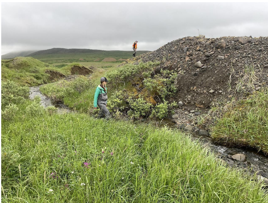
Photograph 3. Dowry Creek (downstream view) where the stream is actively eroding overburden piled next to the creek.
