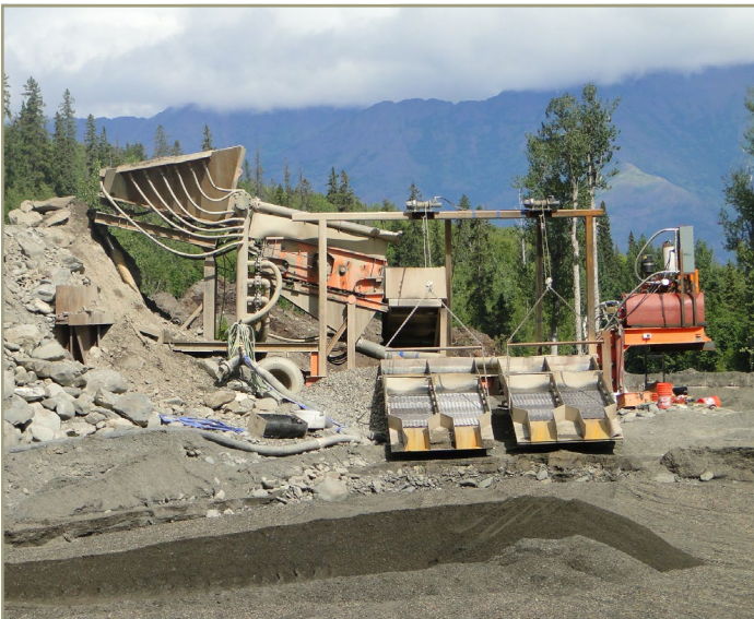
Photo 20. Shaker wash plant, Hope Mining District 2012 (DEC).
