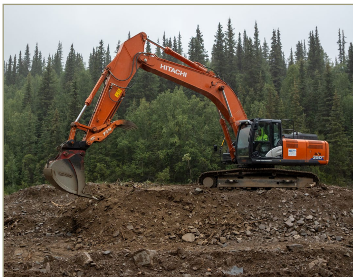
Photo 17. An excavator with a “thumb” is especially useful to pick up and place boulders and logs that are difficult to move with the bucket alone (source unknown).
