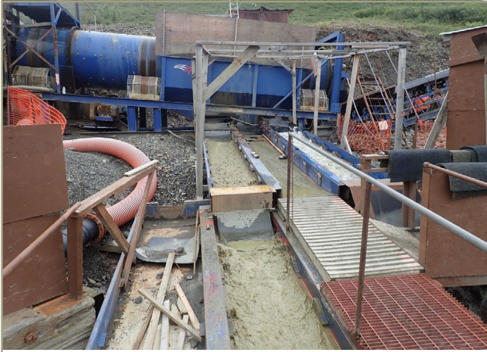
Photo 25. Water flowing through sluice boxes, Valdez Creek Mining District Alaska 2022 (DNR).
