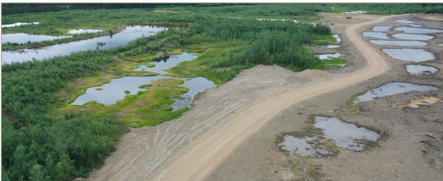
Photo 37. The picture shows stable ongoing operations and successful reclamation of a previously mined area. The area to the right of the road shows ongoing reclamation, with a series of connected ponds and depressions with irregular shorelines and depths to reclaim different aquatic features. Immediately left of the road shows a previously mined area that has been reclaimed with irregular shorelines, depths, and islands to create varying habitats and has excellent revegetation rates of the mined area (USACE).
