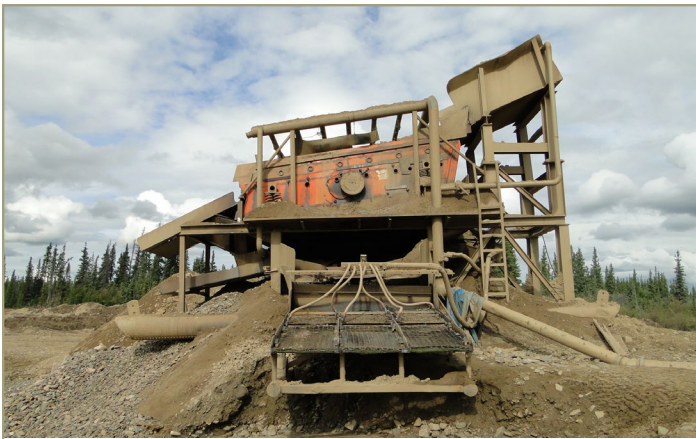
Photo 22. Shaker wash plant with grizzly bars on top, Circle Mining District 2011 (DEC).
