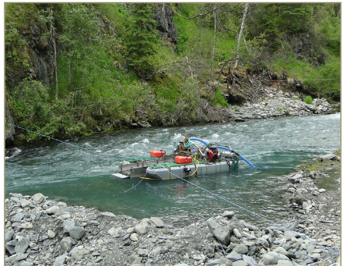
Photo 32. 8" medium-size suction dredge, Hope Mining District, 2012 (DEC).
