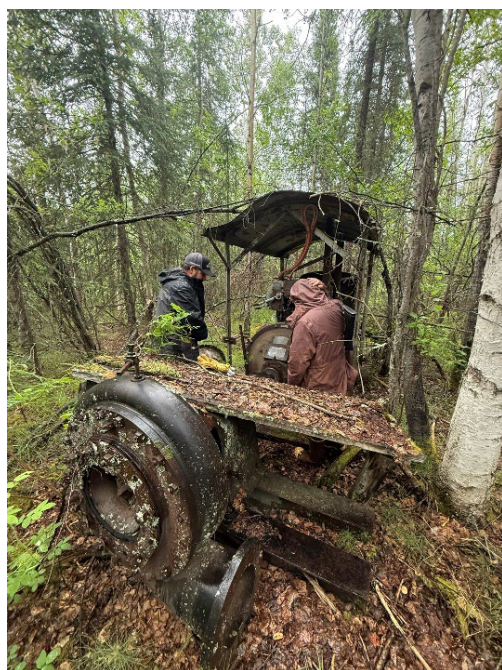
Figure 10. A BLM physical scientist and volunteer document a circa 1916 Murphy diesel engine that was used for historic mining operations in the Ruby Mining District, Alaska. BLM Photo.
