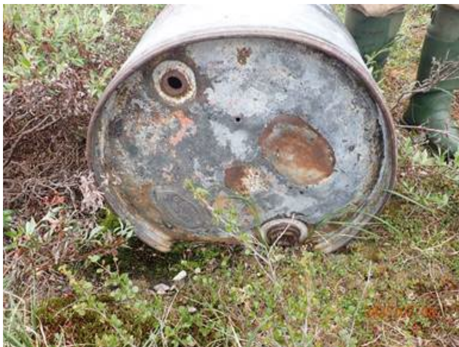
Figure 2. 55-gallon Union Oil Co drum from a US Navy Seismic camp between 1944-1953. The drum style dates to approximately 1912 and exhibits signs of repair and reuse—an uncommon find among the thousands of drums throughout the NPR-A. BLM Photo.
