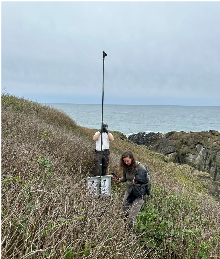
Bat Conservation International and BLM staff install an ultrasonic acoustic detector on Yaquina Head
