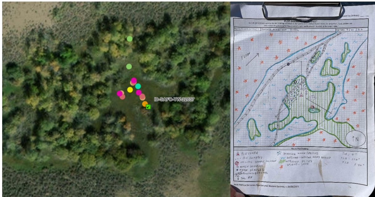
Figure 4. Aerial imagery of a plot from the Data Review Dashboard alongside the plot drawing. The Sample Location (Green Checkbox) is directly on top of the Field Visit (blue star, hidden), with the Site Evaluation form nearby (Orange dot). The plot center (yellow dot for Plot Characterization) is roughly centered amongst the pink LPI transect starts (pink dots). Soil pit (teal) and water quality (green dot) are in locations that match those shown in the plot drawing.
