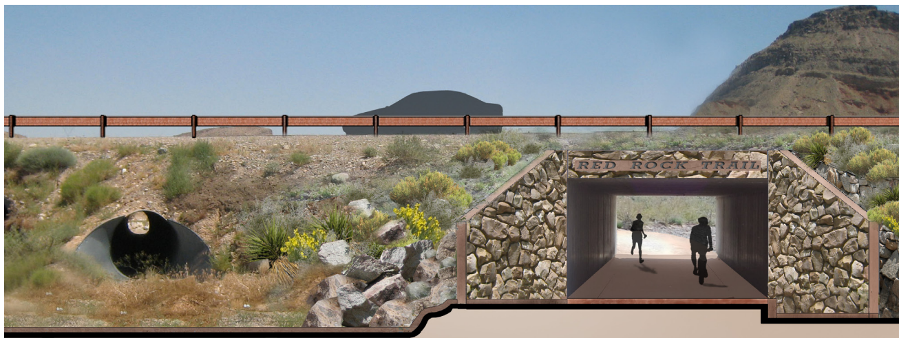
Illustrative cross section of proposed underpass near the visitor center
