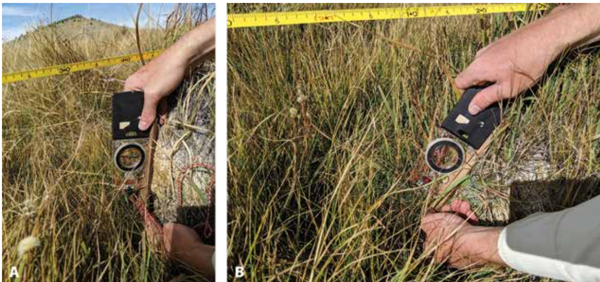
Figure 42. Measuring slope of the leading edge with a ruler and compass, showing (A) a steeper side slope and (B) a moderately shallow side slope.
