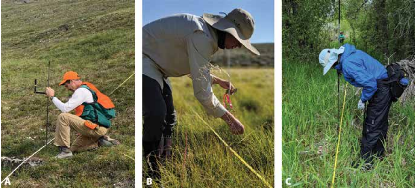
Figure 32. Examples of line-point intercept data collection areas along transects with either (A) a mounted laser setup or (B and C) pin flags.
