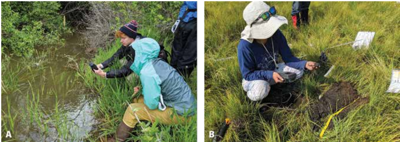
Figure 48. Measuring pH, specific conductance, and temperature with a water quality probe in (A) surface water and (B) groundwater within a soil pit.
