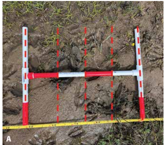
Figure 52. Soil alteration is evaluated by projecting five lines (red dashed lines) across the frame and perpendicular to the center bar. Two lines coincide with the outer cross pieces of the frame, and three inner lines are spaced 12.5 cm apart. In this example, soil alteration would be recorded as 4 because the first, second, third, and fourth lines intersect soil alteration. The second and third lines both intersect the same large hoofprint.
