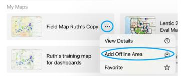
a. This will open a window to adjust the frame and level of detail you want in your downloaded map. The higher the level of detail, the smaller the area you can download, as indicated by the black box that will appear on the map.
