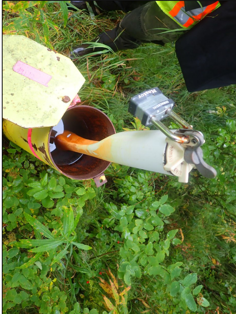
Photograph 2-2. MW12, frost jacked with collapsed PVC. 22 August 2022.
