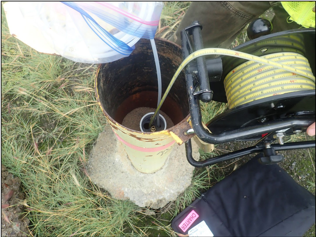
Photograph 2-9. MW10 well gauging. 22 August 2022.
