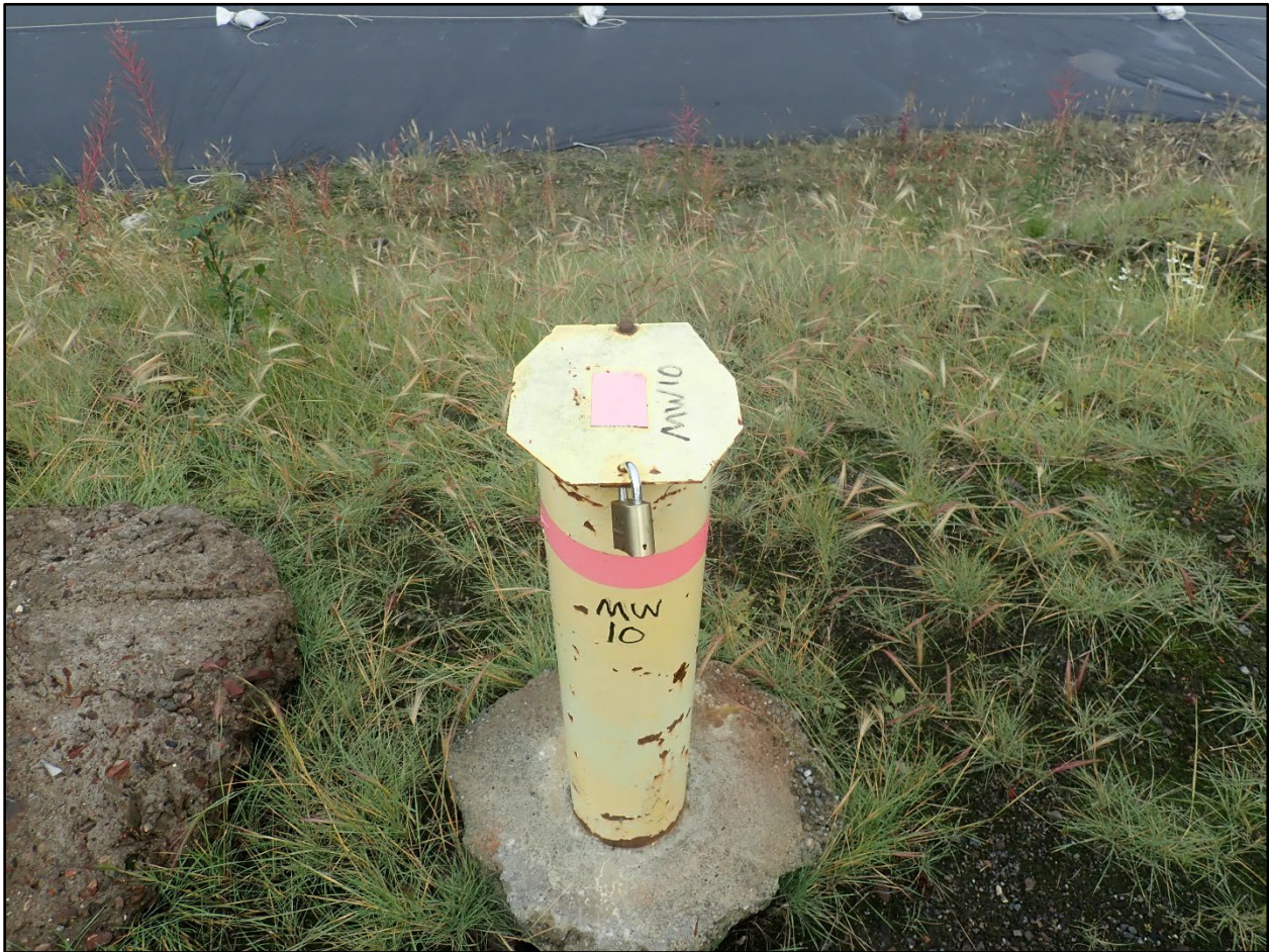
Photograph 2-10. MW10 settling around concrete base August 2022.
