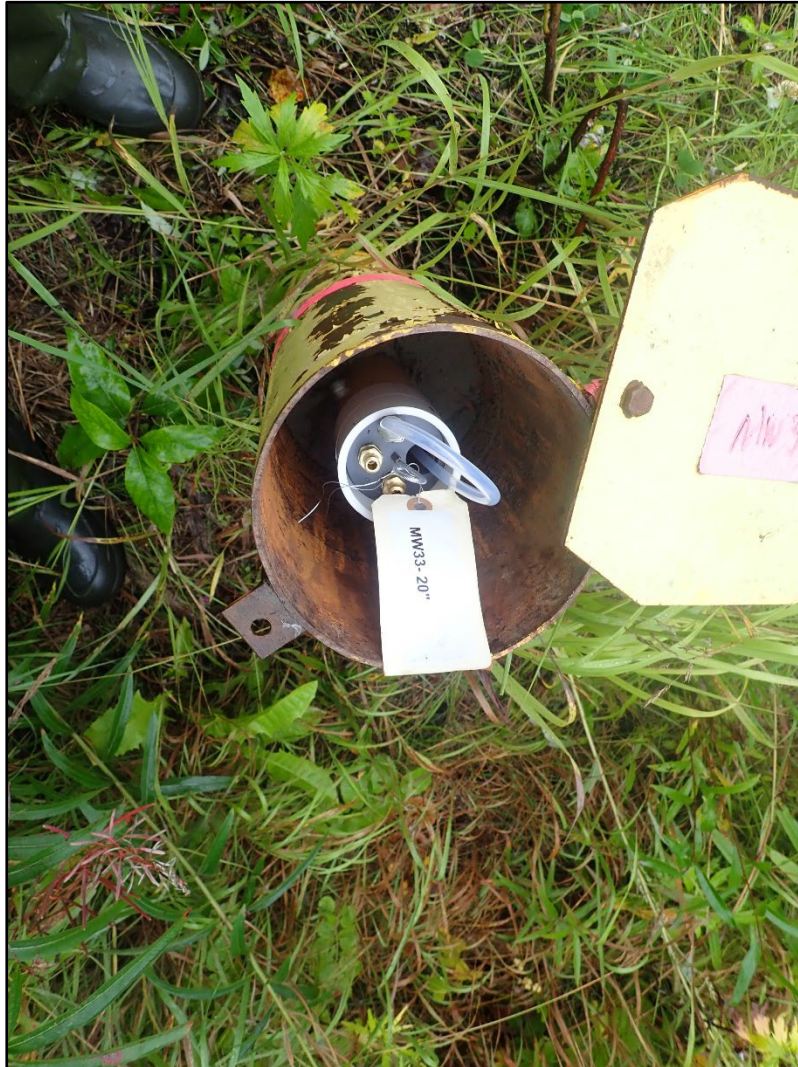
Photograph 2-1. MW33 with new bladder pump system installed 22 August 2022.
