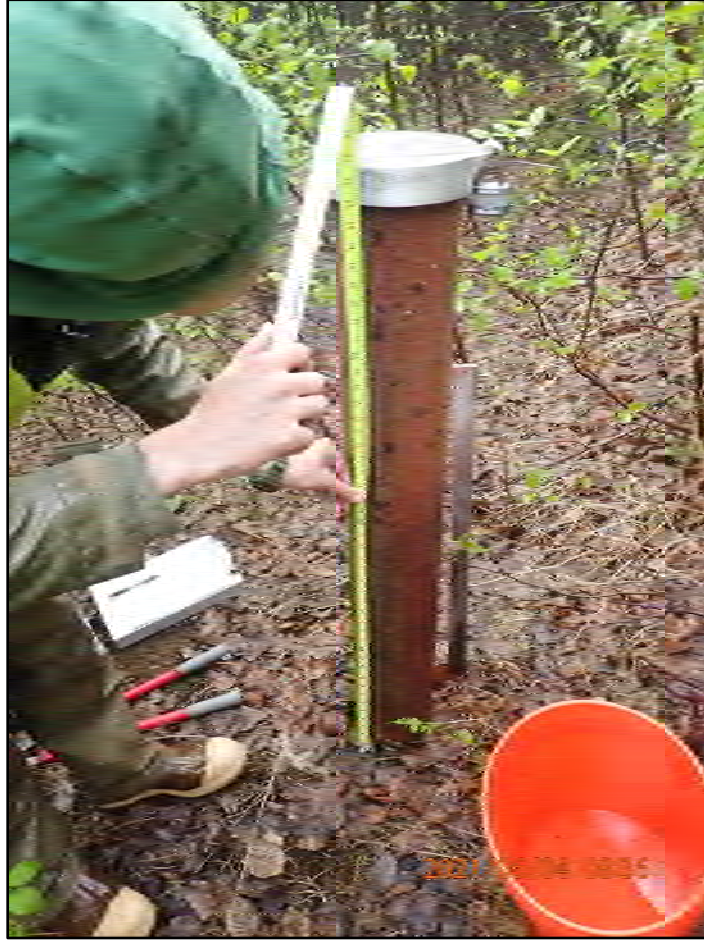
Photograph 2-5. MW35, measuring stickup of monument. June 4, 2021.
