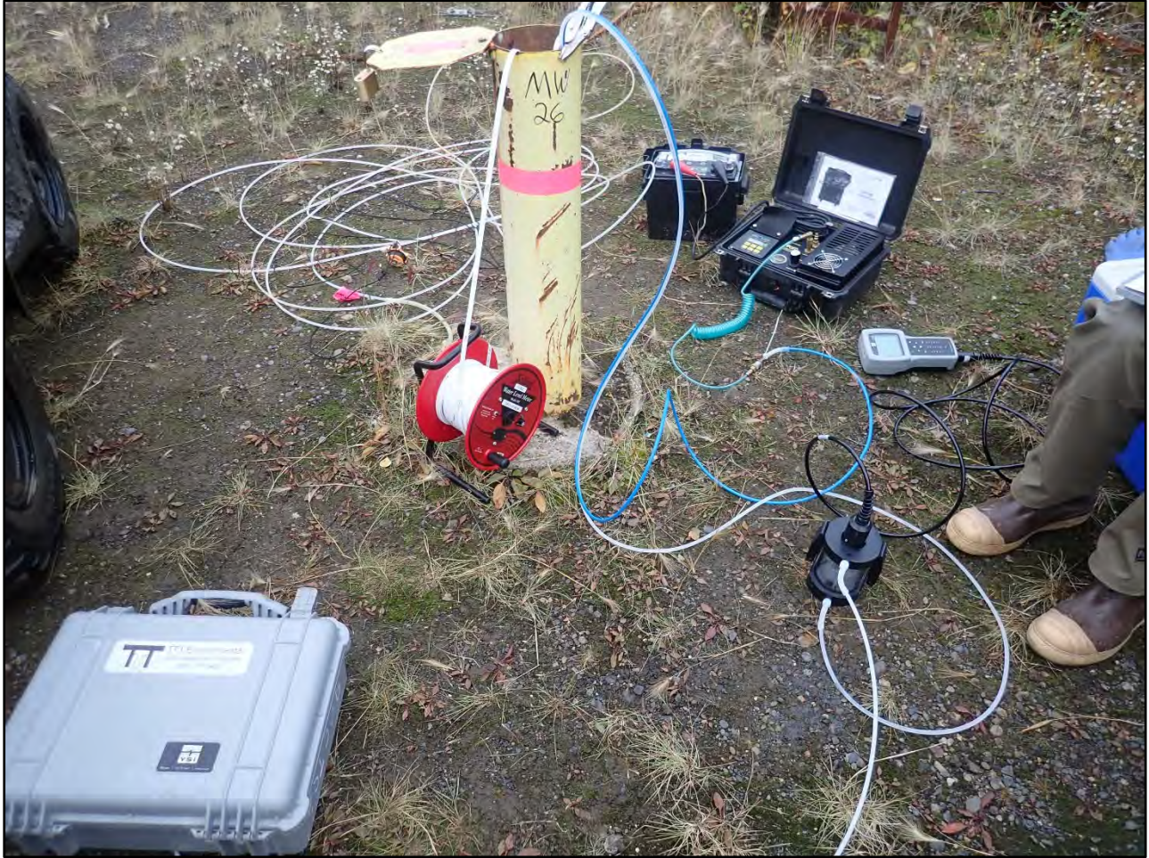
Photograph 2-18. MW26, groundwater sampling setup. August 30, 2021.
