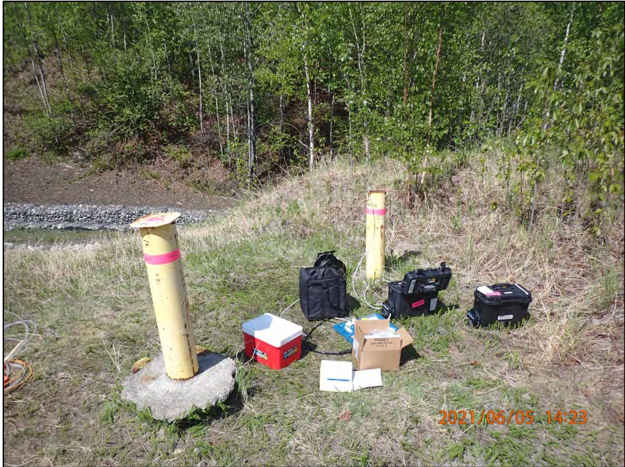
Photograph 2-6. MW16 and MW17, groundwater sampling with peristaltic pump. June 5, 2021.
