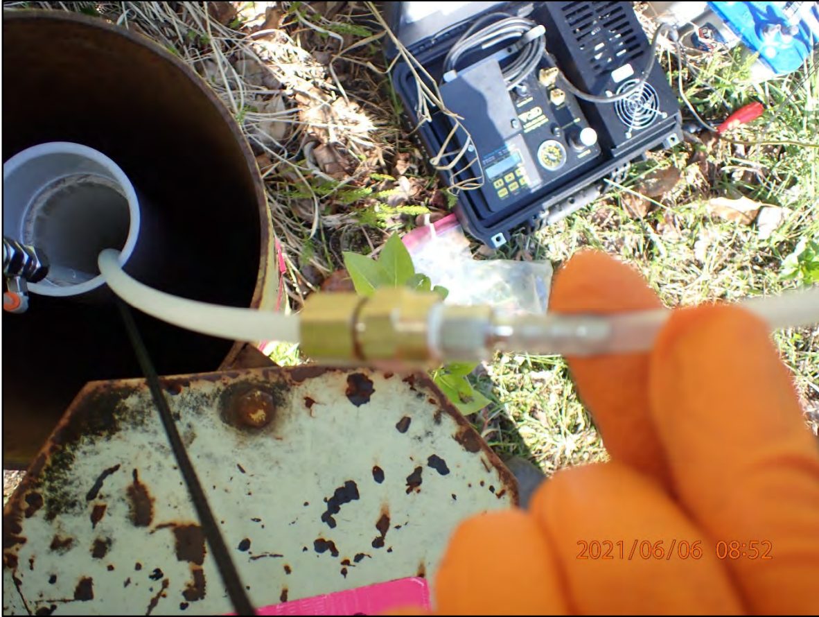
Photograph 2-13. MW42, splice that failed. June 6, 2021.
