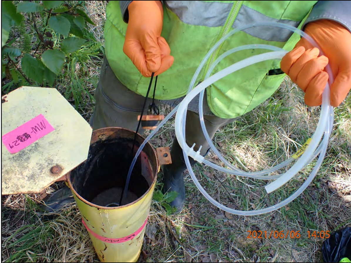
Photograph 2-12. MW29, missing air tubing. June 6, 2021.
