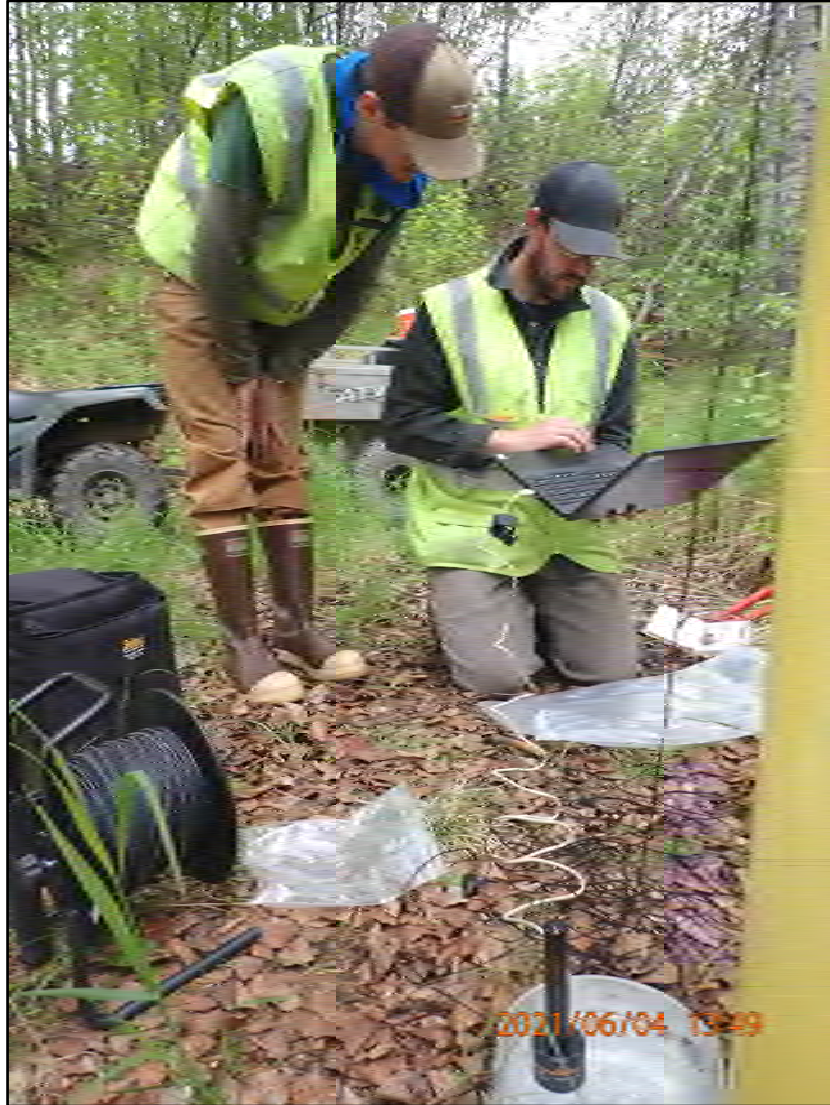
Photograph 2-11. MW56 downloading a transducer. June 4, 2021.
