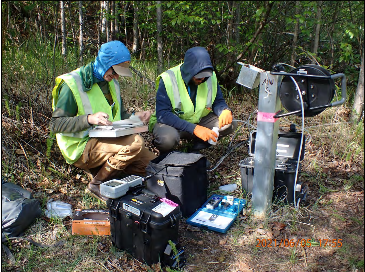
Photograph 2-7. MW06 groundwater sampling with a peristaltic pump. June 5, 2021.
