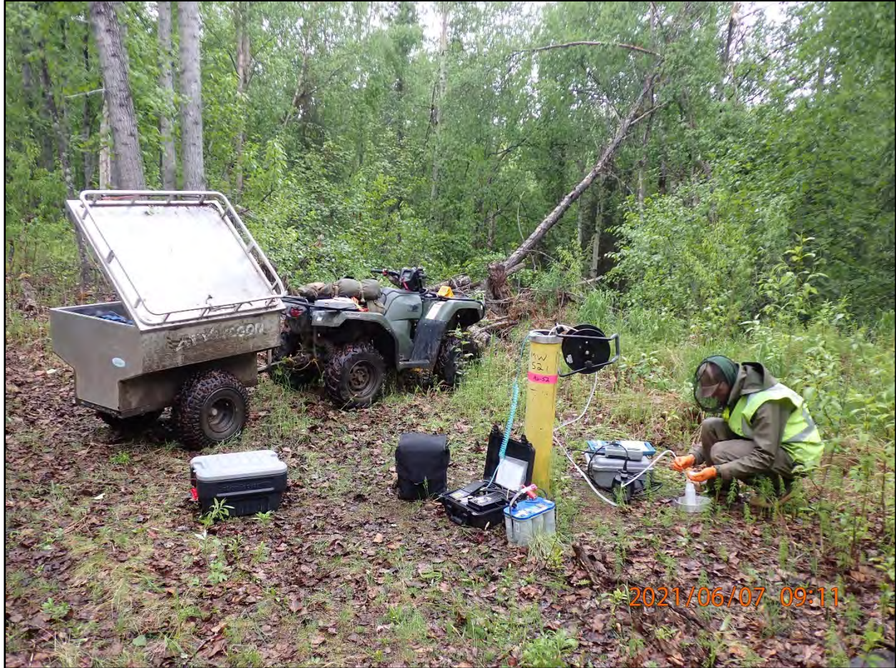
Photograph 2-8. MW52 groundwater sampling with a bladder pump and controller. June 7, 2021.
