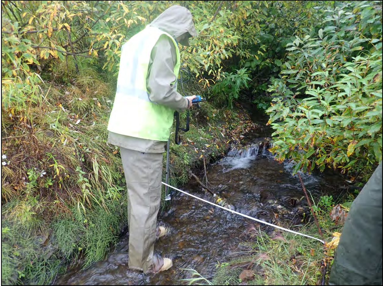
Photograph 2-21. RD08 collecting stream discharge measurements. September 3, 2021.
