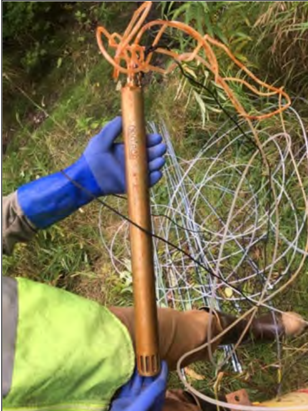
Photograph 2-15. MW29, Precipitate staining and silt on pump after retrieval, but prior to tubing replacement. August 30, 2021.
