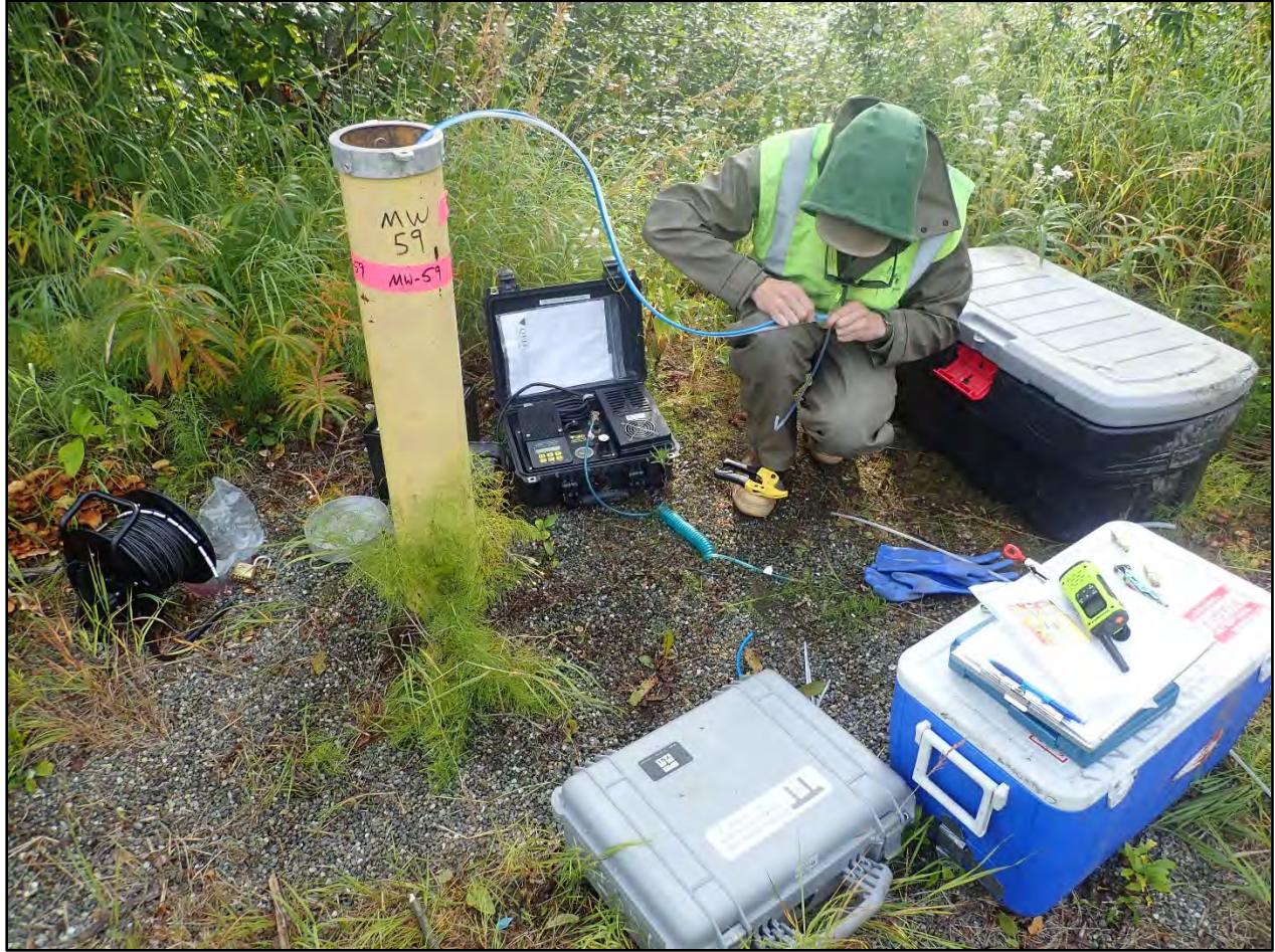
Photograph 2-25. MW59 setting up new tubing after replacement. September 1, 2021.
