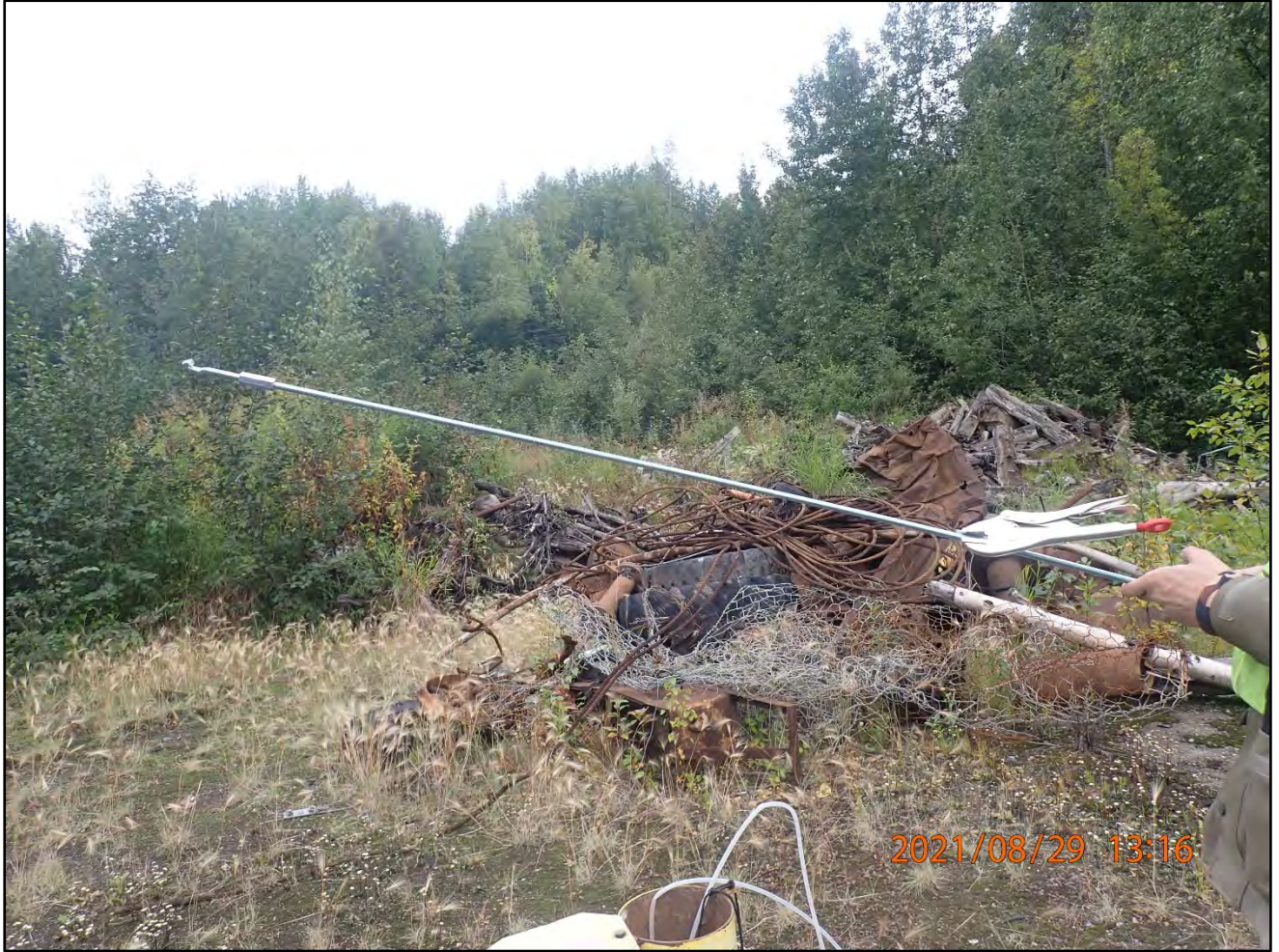
Photograph 2-17. Pump Retrieval tool used to pull MW-29. August 29, 2021.
