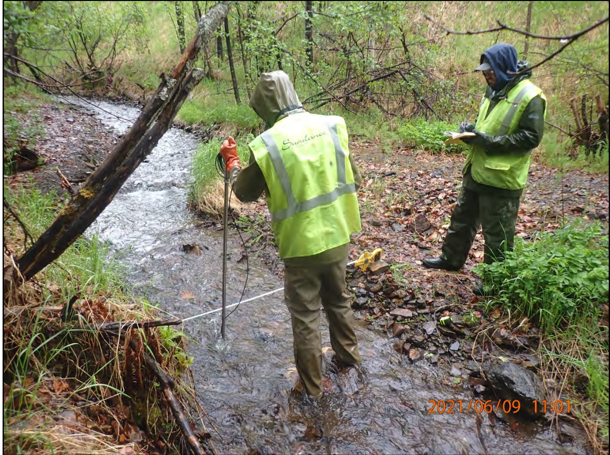
Photograph 2-9. RD06SW stream gauging. June 9, 2021.
