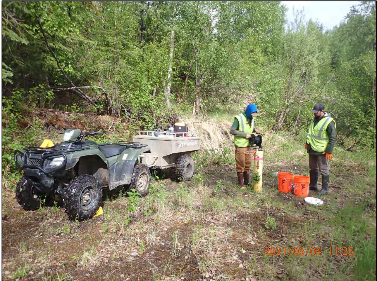
Photograph 2-4. MW43, measuring depth to groundwater. June 4, 2021.
