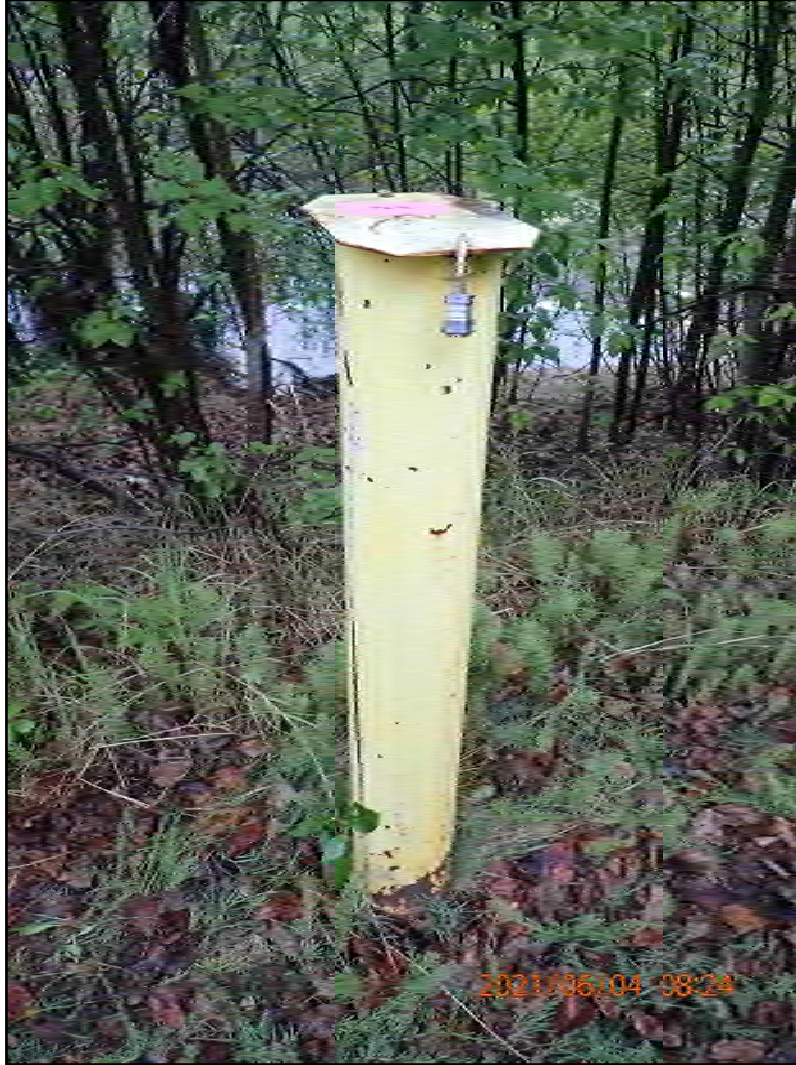
Photograph 2-1. MW09, closed, locked, and labeled. June 4, 2021.
