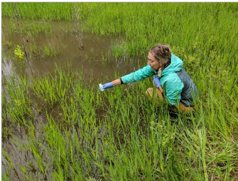
Figure 46. Two methods for collecting a water quality grab sample in riparian and wetland environments: (A) collecting the sample by hand in flowing water and (B and C) collecting the sample using a long-handled dipper.
