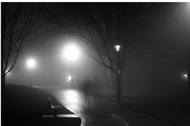
Glare from direct view of light sources and reflection from wet pavement.
