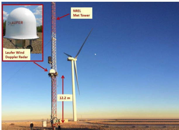
An ADLS radar unit mounted on a meteorological tower at a wind energy facility.
