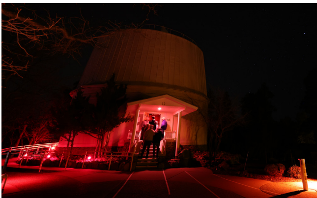
The pedestrian path to the Lowell Observatory uses “night sky friendly” amber path lighting.
