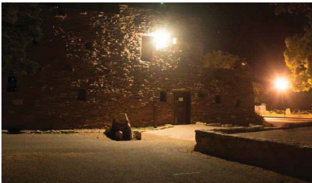
These horizontally aimed floodlights cause skyglow, light trespass, and glare.
