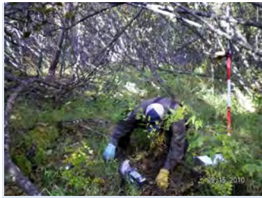
Surface soil sampling for XRF field screening.
