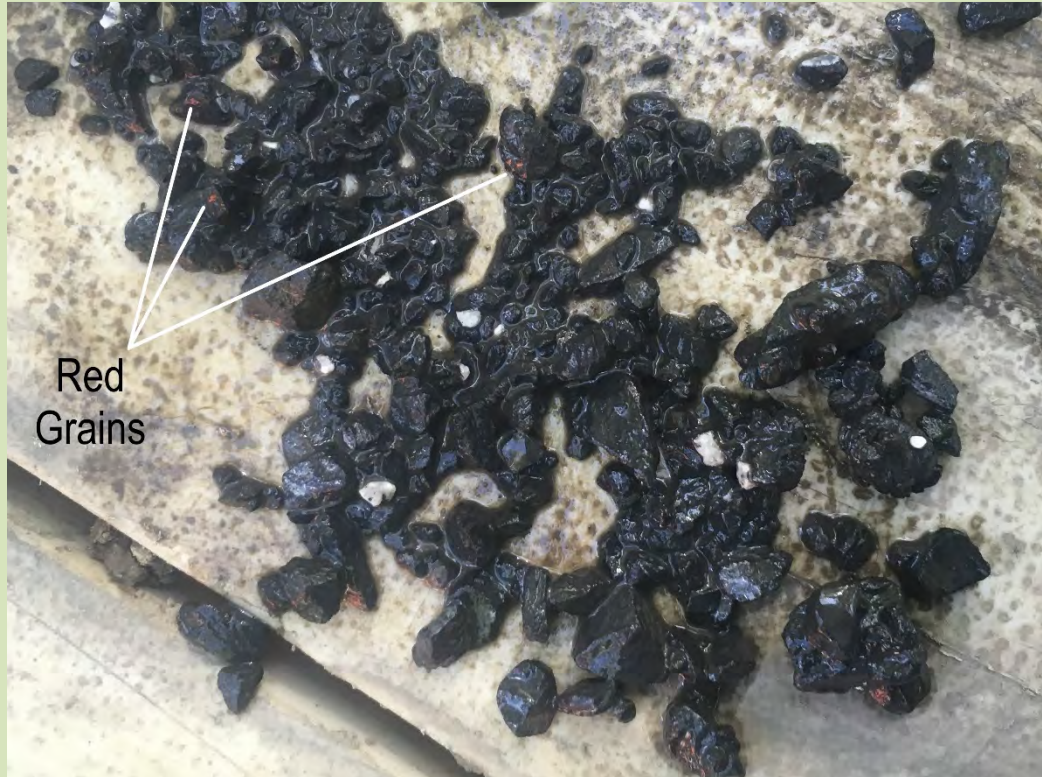
Photograph 6. Drill cuttings from borehole SM78 (monitoring well MW50) from depth interval 72.5 to 75 feet bgs.
