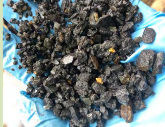
Photograph 5. Drill cuttings from borehole SM70b (monitoring well MW42) from depth interval 127 to 128 feet bgs. Note orpiment (the orange grains).
