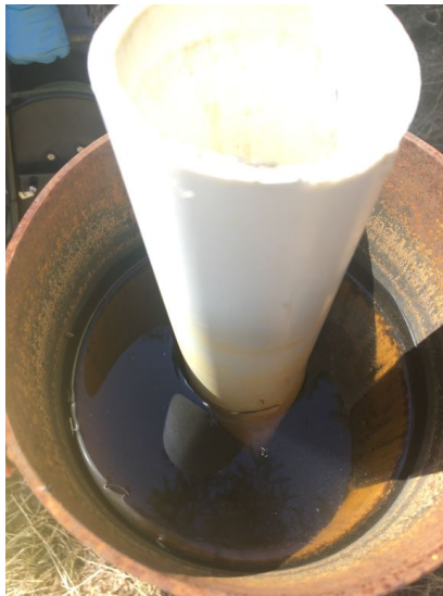
Photo 3: Bent inner casing of MW12 as a result of frost-heaving.
