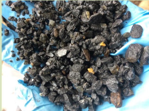
Photograph 2 Drill cuttings from borehole SM70b from depth interval 127 to 128 feet bgs. Note orpiment (bright orange grains).
