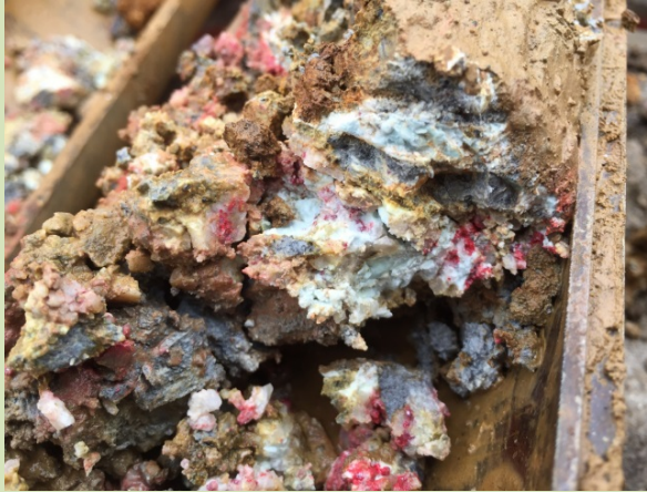
Photograph 1 Weathered bedrock in split spoon sampler from depth interval 44 to 45 feet bgs, borehole MP098. Note cinnabar (red grains).
