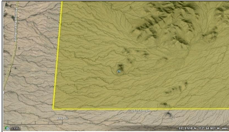
Figure 4 – A PLSS boundary is optimal in a landscape such as this where there are no clearly definable permanent natural or human-made features. As seen above, numerous minor dry ambulatory washes cut across unconsolidated (non-bedrock) material. Had one of the washes been selected as the southern boundary, it could move or become indistinguishable, making it very difficult to develop a legal boundary description or to manage the boundary to prevent incursions.
