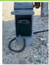
Pneumatic vehicle counter and housing
